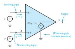
Problem 6 The actual op amp is a five-terminal device. After reconciling this issue of the vanishing terminal in the previous problem, give an expression for the nodal output voltage with respect to  $V_{SS}$  for the operational amplifier shown below which explicitly shows the 5 terminals of the device.
